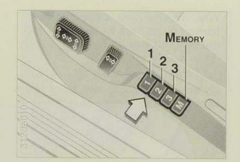
Three different seat, outside mirror and (only with electric steering wheel adjustment) steering wheel positions can be memorised.
