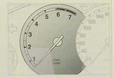
Never allow the engine to run in the red zone of the revolution counter.
