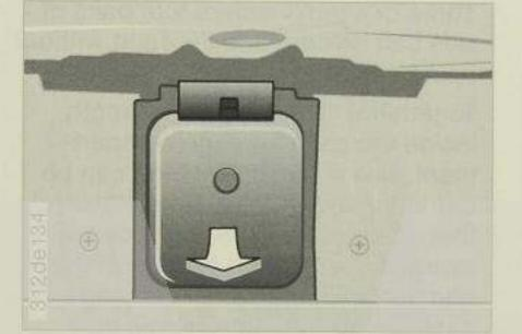
From the luggage compartment side, attach the cover flap to the underside of the rear-window shelf with the magnetic holder provided.
