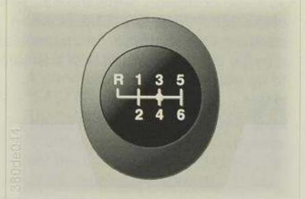
The normal rest position for the gear lever (marked by a dot) is in the 3rd/ 4th gear plane of the gate.
