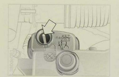
Coolant level with engine cold (app. 20°C):
