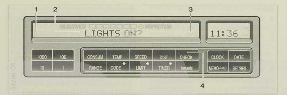
System malfunctions are shown in plain Priority 1 text, and a gong warning sounded. There is also a general warning light on the instrument panel which comes on during the journey if a fault signal is present.
