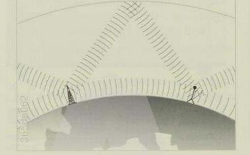
The MW, LW and SW wavebands can be heard a long way from the transmitter, because the signals spread out both as ground waves and through the air, reflected by the ionosphere.
