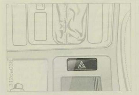
The pushbutton lights up in a regular rhythm when the hazard warning flashers are operating.
