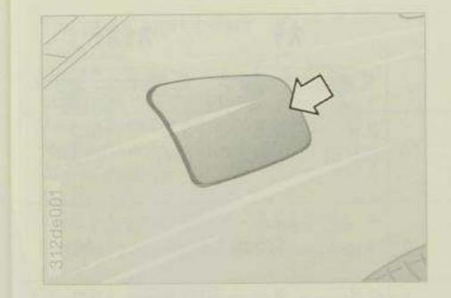
To open the fuel filler flap, press the front end in so that the flap can be lifted.
