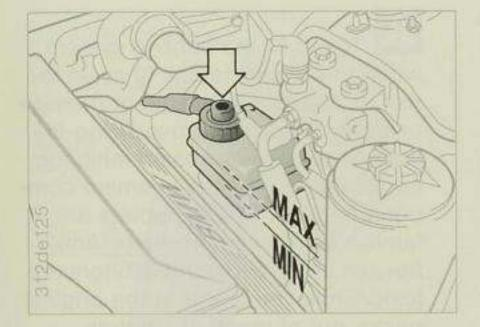
Fill to the upper MAX mark (level can be checked from the outside).
