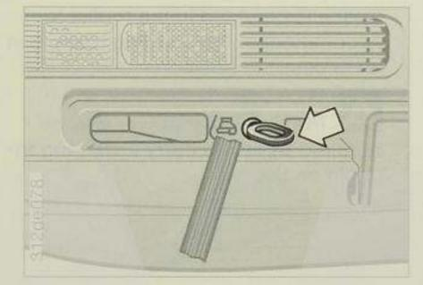
The screw-in towing eye is kept in the toolkit and must always be carried. It can be attached to the car at the front or rear.
