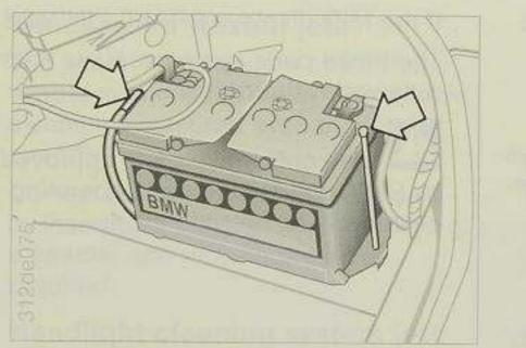
The two batteries are located behind the side trim panels in the luggage compartment. There is a positive terminal connection in the engine compartment, to which a jump-start lead can be attached if necessary (see Page 110).
