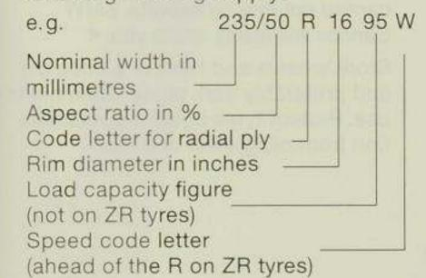
The speed code letter indicates the maximum permissible speed at which the tyre is to be operated.
