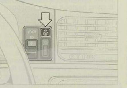
Press the button: When the telltale light is on, the heated rear window is operating at full heat output (rapid demisting).
