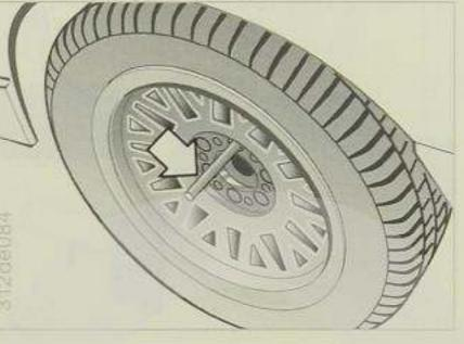
12 Centre the wheel stud cover and attach. Push it on and turn to the left or right until wheel cap locks into place. Cross-spoke wheels: align with the arrow marked on the wheel stud cover with the line marked on the wheel and push on the wheel cover.
