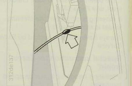
Before taking off the right-hand luggage compartment side trim, separate the plug connector for the manual fuel filler flap release at the cable (arrow).
